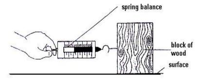
The amount of force required to move the block of wood are shown in the table below.
