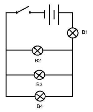
All the light bulbs light up when the switch is closed. If bulb 3 (B3) fuses, which of the following light bulbs will still light up?
