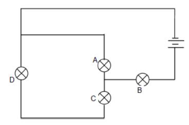
Which bulb(s) will light up when bulb **D** fuses?
