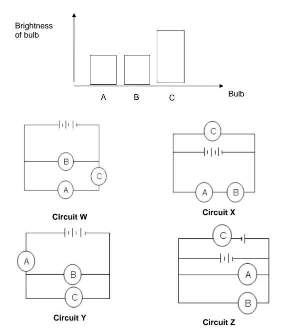
Which of the above circuits, W, X, Y or Z correctly represents the graph shown?
