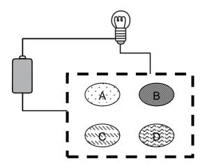
The objects were connected to see if the bulb can light up.
